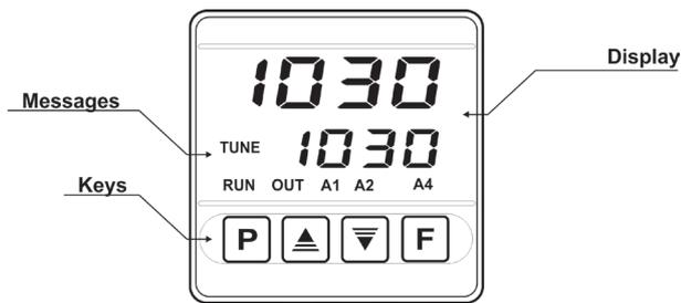
Fig. 02 – Front panel
