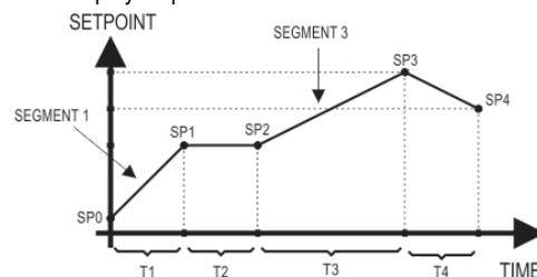
**Fig. 03** - Example of a Ramp and Roak
