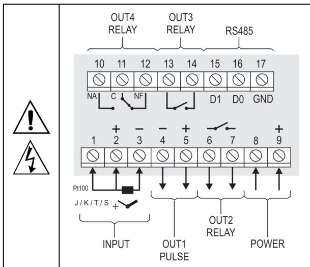
**Fig. 01** - Inputs, outputs and power supply connections
